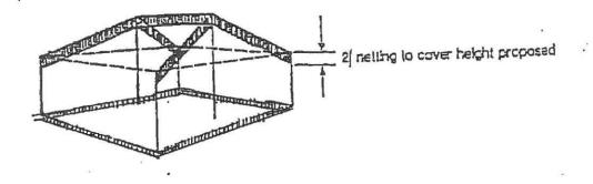
Netting must be placed at the height proposed for any building pad as shown above. The structure height netting must be placed to include the height of the building plus the height of the pad. All heights shall be measured from the existing grade or elevation prior to any grading or alteration of the site.
