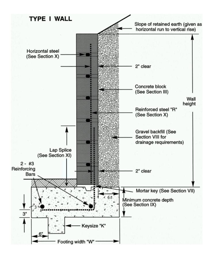
NOTE: The bottom leading edge of all retaining wall footings shall be 7'-0" minimum from FACE of slopes where the ground slopes away from the wall.
