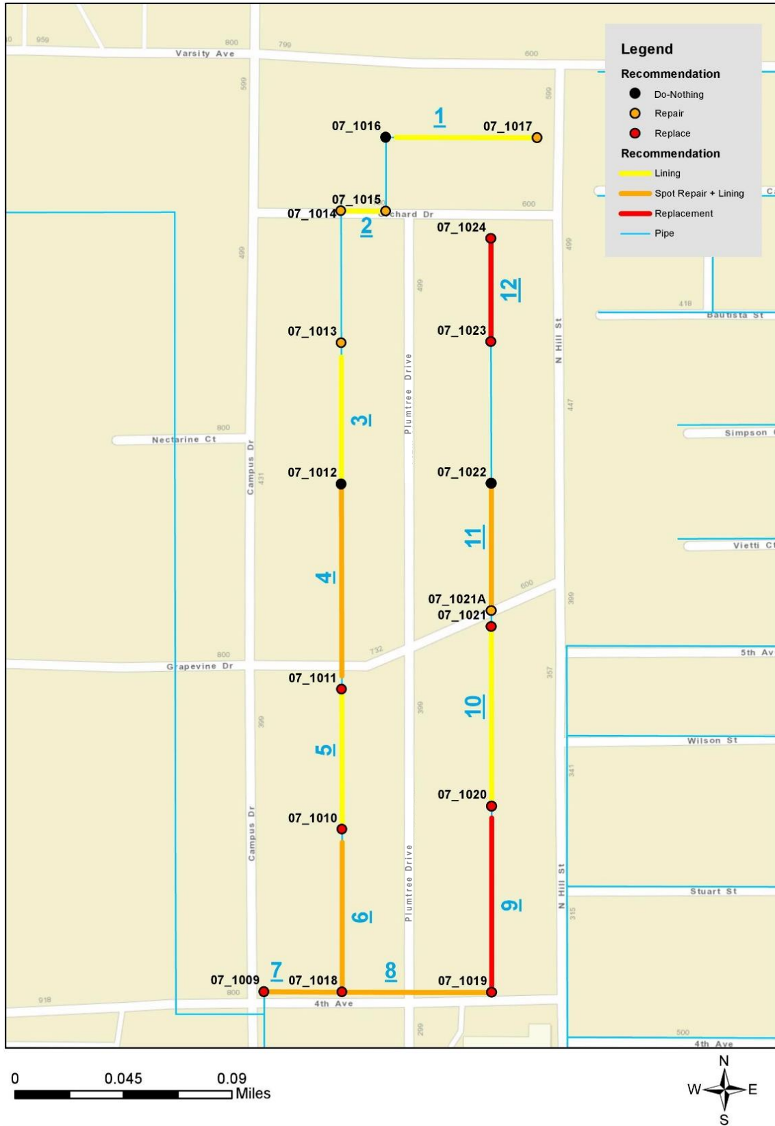
Figure 7.12 – Extent of Plumtree Drive Alleys Pipeline Project
