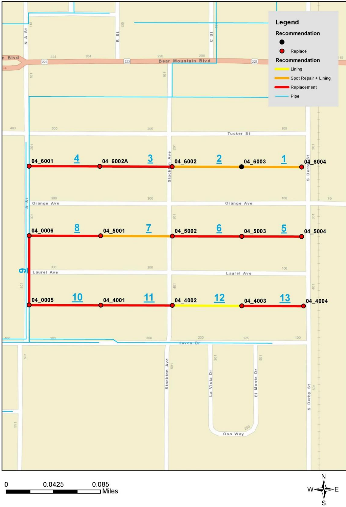
Figure 7.4 – Extent of A Street Pipeline Project
