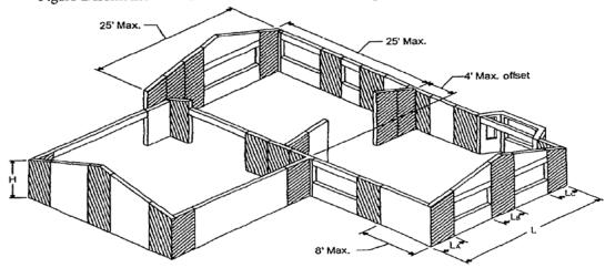
Minimum length of wood structural panel walls.
