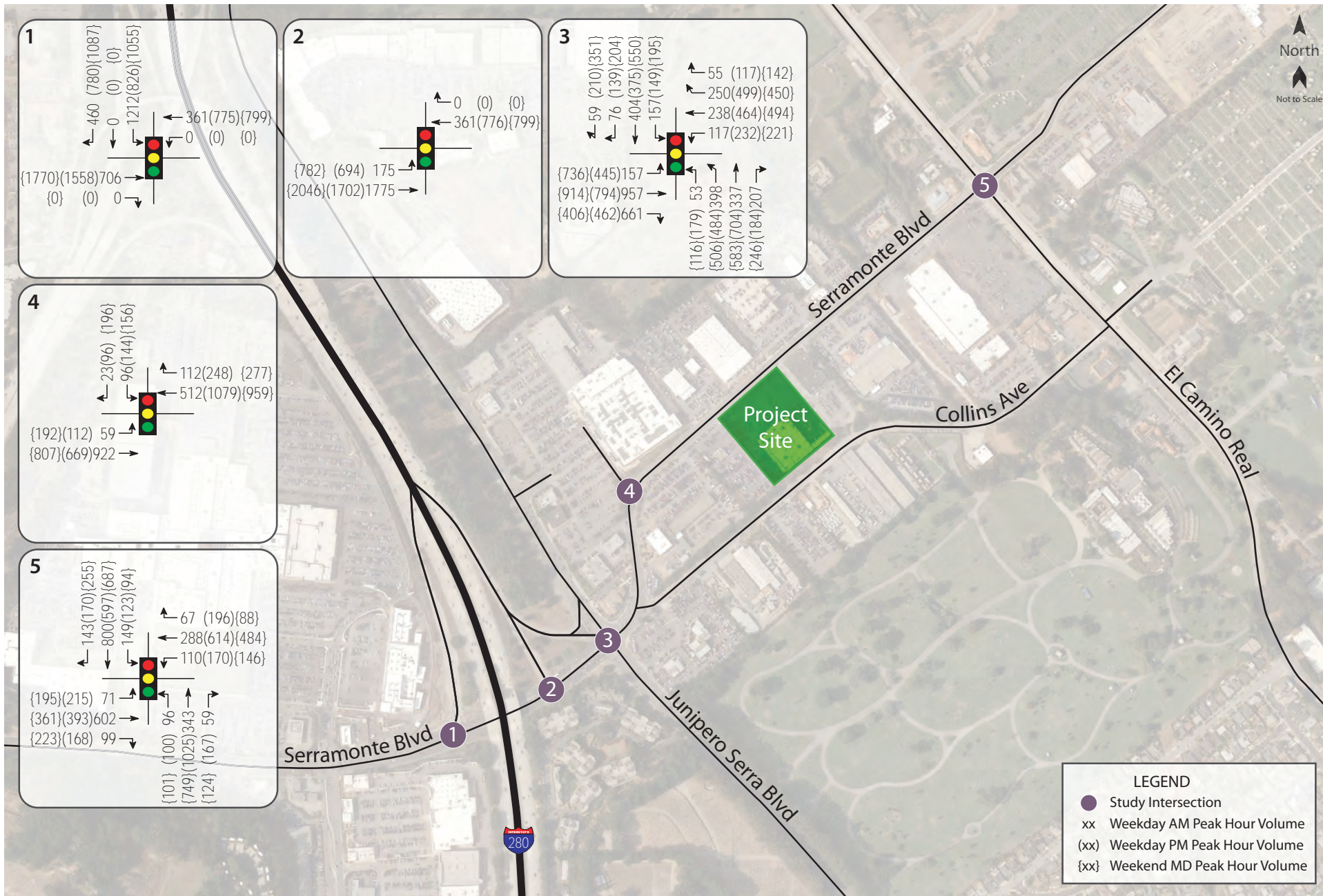
Traffic Study for the 775 Serramonte Boulevard Cadillac Dealership Figure 3 – Future Traffic Volumes
