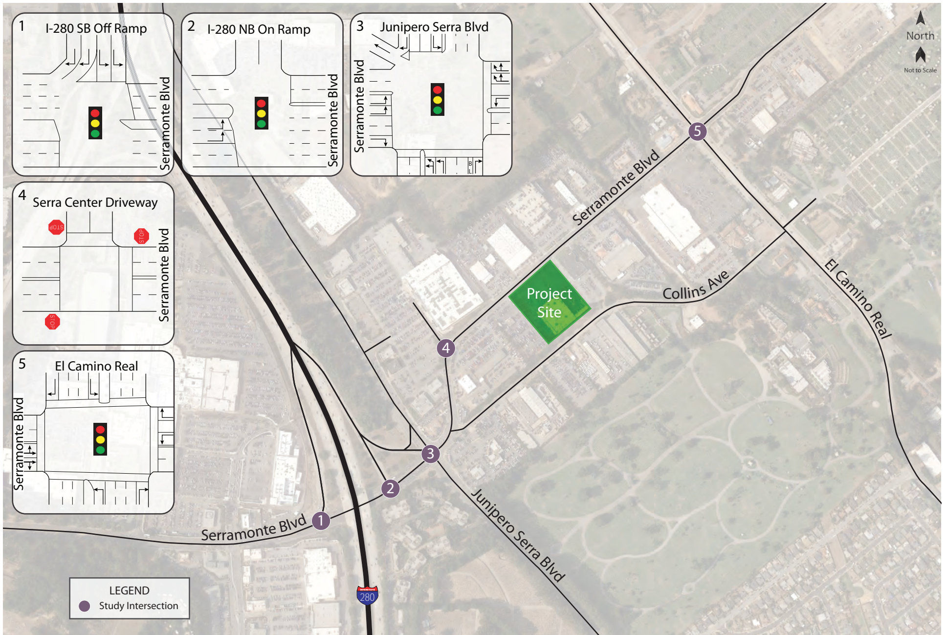
Traffic Study for the 775 Serramonte Boulevard Cadillac Dealership Figure 1 – Study Area and Existing Lane Configurations
