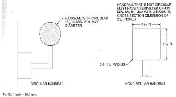
Figure R311.7.8.3(1) TYPE 1 HANDRAIL
