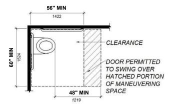
FIGURE 11B-604.3.1 - SIZE OF CLEARANCE AT WATER CLOSETS
