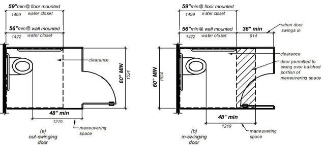
FIGURE 11B-604.8.1.1.3 - MANEUVERING SPACE WITH END-OPENING DOOR
