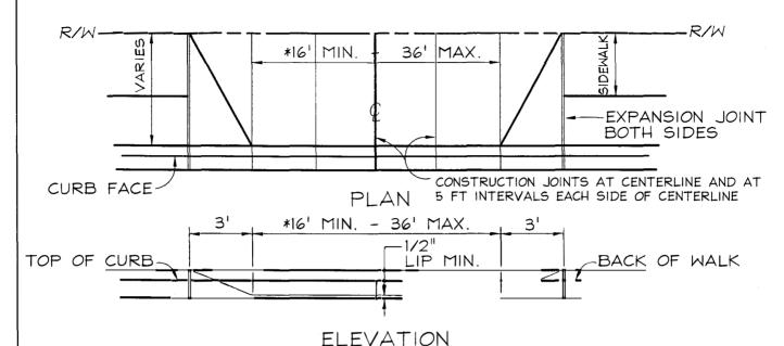
\*MIN. DRIVEWAY WIDTH OF 30' FOR TWO-WAY TRAFFIC. REDUCED DRIVEWAY WIDTHS MAY BE USED WITH APPROVAL BY THE CITY ENGINEER.
