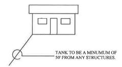
TANKS TO BE CONSTRUCTED OF MOLDED PLASTIC, FIBERGLASS, OR GALVANIZED STEEL, NOT LESS THAN 12 GAUGE.
