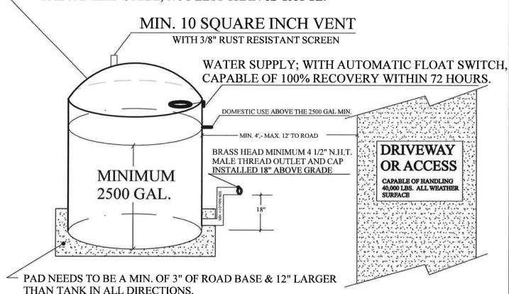
LOCATION: TANK NOT LESS THAN 50' FROM STRUCTURE. NOT LESS THAN 4' NOR MORE THAN 12' FROM ROADWAY, READILY ACCESSIBLE FOR FIRE APPARATUS. MINIMUM 8' FROM FLAMABLE VEGETATION. REFLECTIVE BLUE SPHERE MOUNTED WITH ADDRESS NUMBERS TO IDENTIFY TANK.
