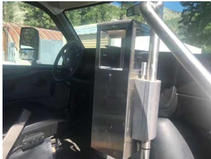
Farebox mounted in cutaway bus.
