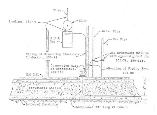
SECTION 250.52 (3) Concrete-Encased Electrodes. A concrete-encased electrode shall consist of at least 6.0 (20 feet) of either (1) or (2).
