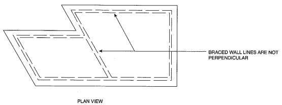
FIGURE 2308.12.6(7) BRACED WALL LINES NOT PERPENDICULAR
