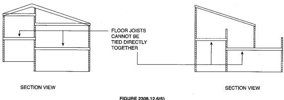
FIGURE 2308.12.6(6) PORTIONS OF FLOOR LEVEL OFFSET VERTICALLY
