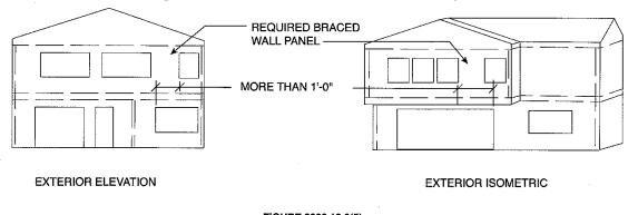
FIGURE 2308.12.6(5) BRACED WALL PANEL EXTENSION OVER OPENING
