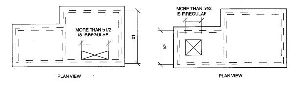
FIGURE 2308.12.6(8) OPENING LIMITATIONS FOR FLOOR AND ROOF DIAPHRAGMS
